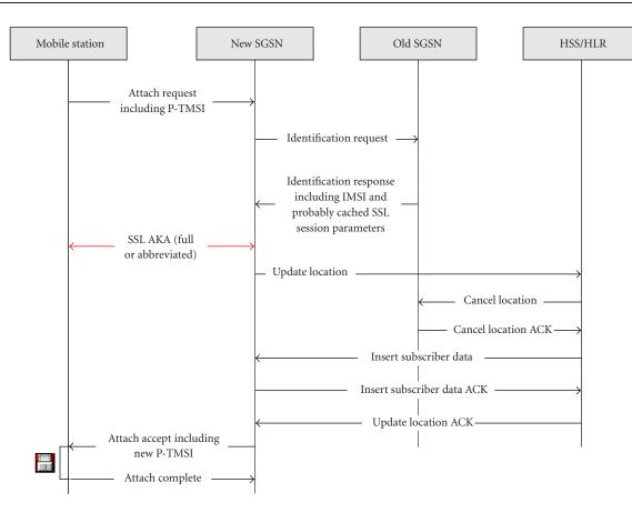
FIGURE 5: MS's attach procedure.
