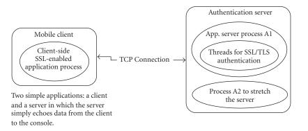
FIGURE 8: Software architecture.
