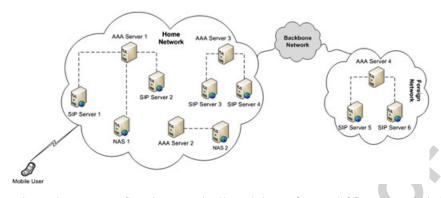
Figure 4. Accounting system configuration supporting Network Access Server and SIP servers as AAA clients.
