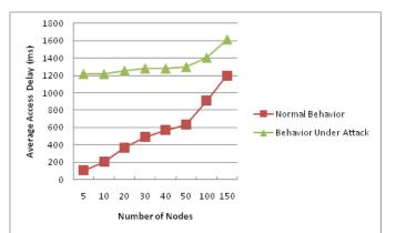
Fig. 11. Average access delay in msec for a different number of contending nodes
