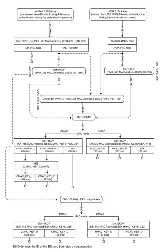
Fig. 3. Complete Message Exchange and Key Derivation
