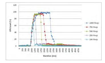
Fig. 13. System CPU load during an Auth-Req Attack
