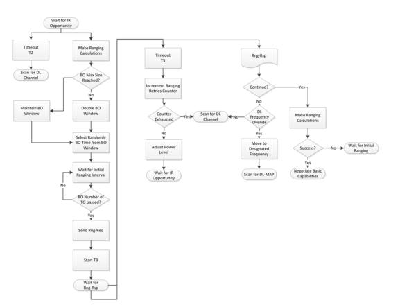
Fig. 2. Flowchart of the Initial Ranging process
