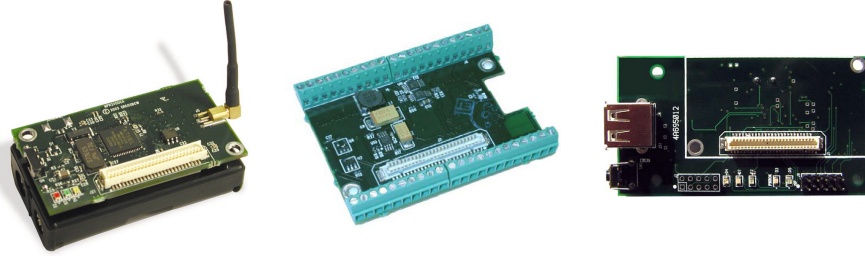
Fig. 3. The hardware platform includes a Mote Processor Radio platform (MPR2400), a data acquisition board (MDA300CA) and a Mote Interface Board (MIB520CA) for network base stations and programming interfaces.
