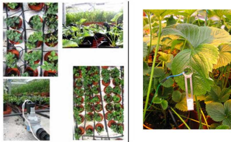
Fig. 14. Experimental setup (left); attaching a thermistor to a strawberry (right)
