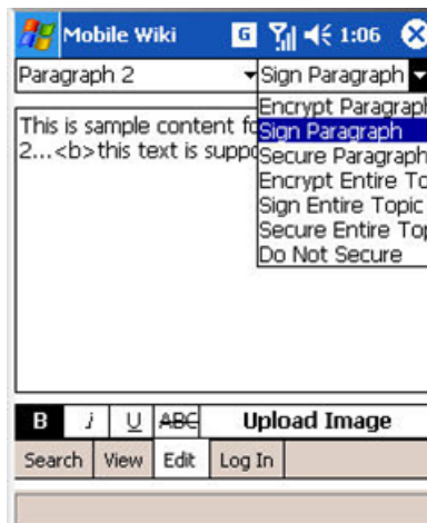
Figure 5. A snapshot of the client wiki application (“Secure” means encrypt + sign)
