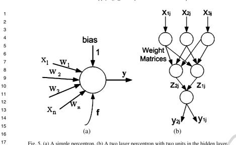
Fig. 5. (a) A simple perceptron. (b) A two layer perceptron with two units in the hidden layer.
