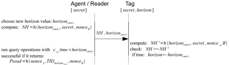
**Fig. 6.** Compact schematic of time Horizon Update
