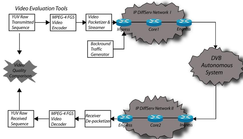
Figure 3.1: Heterogeneous IP/DVB testbed
