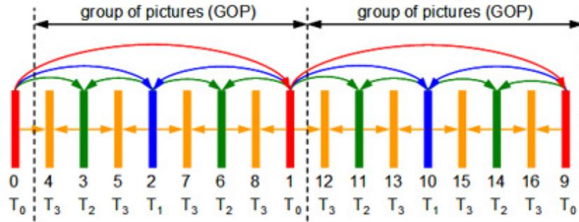
Figure 2.3: Four-level hierarchical-B prediction structure
