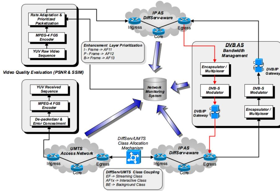
Figure 5.2: Testbed Configuration Setup
