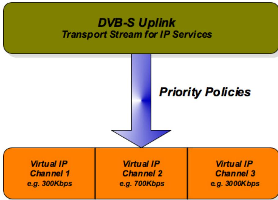
Figure 2.5: Bandwidth slicing principle in a DVB uplink
