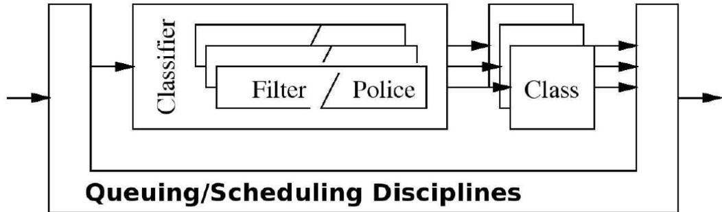
Figure 3.2: Linux DiffServ Architecture
