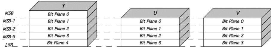
Figure 2.2: The structure of bit planes Y, U, V
