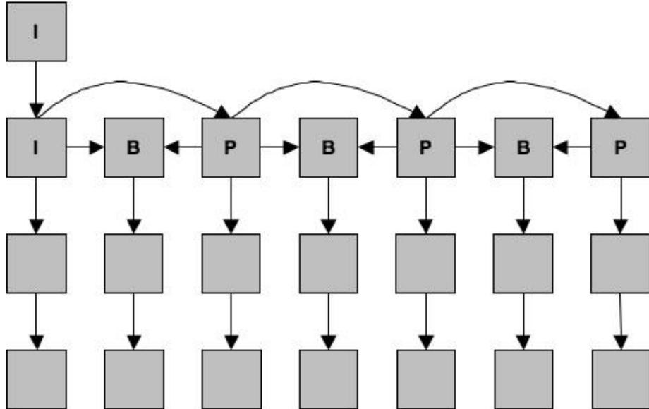
Figure 2.4: A directed acyclic graph captures the decoding dependencies for an SNR-scalable encoding of video with I-frames, P-frames, and B-frames. Squares represent data units and arrows indicate decoding order.
