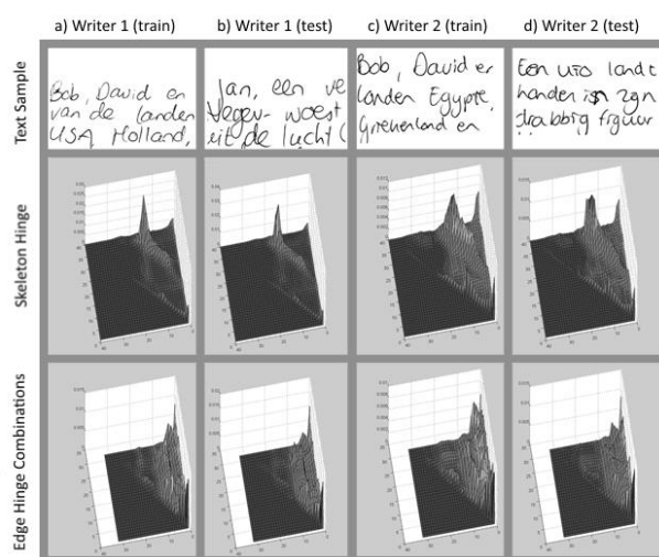
Fig. 6. Text samples from two different writers (train set on left, test set on right) along with skeleton hinge distribution feature surface (middle) and edge hinge combinations feature surface (bottom). The text samples on the top are fragments of the text sample used, and are provided for illustrating the differences of handwriting between those texts.
