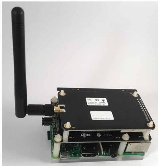
Figure 26 (source in Appendix I): Complete gateway (Raspberry Pi 3 + RAK831)
